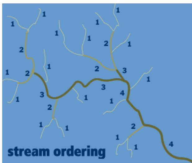
Figure 3.1 Stream Ordering (NRCS) and the Depiction of a Dendritic Stream System
