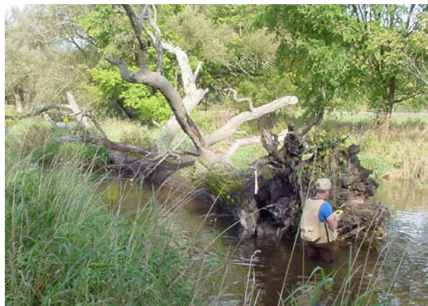
Figure 6.1 Using a hand held GPS receiver to locate a debris jam downstream of South Kortright.
